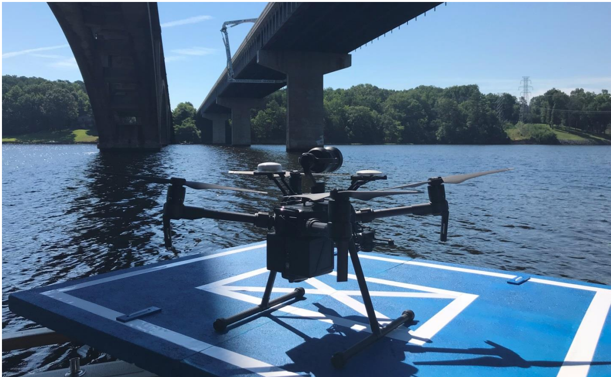
Figure 2. DJI Matrice 210 RTK on Launch Pad with Single Camera Mounted on Top
