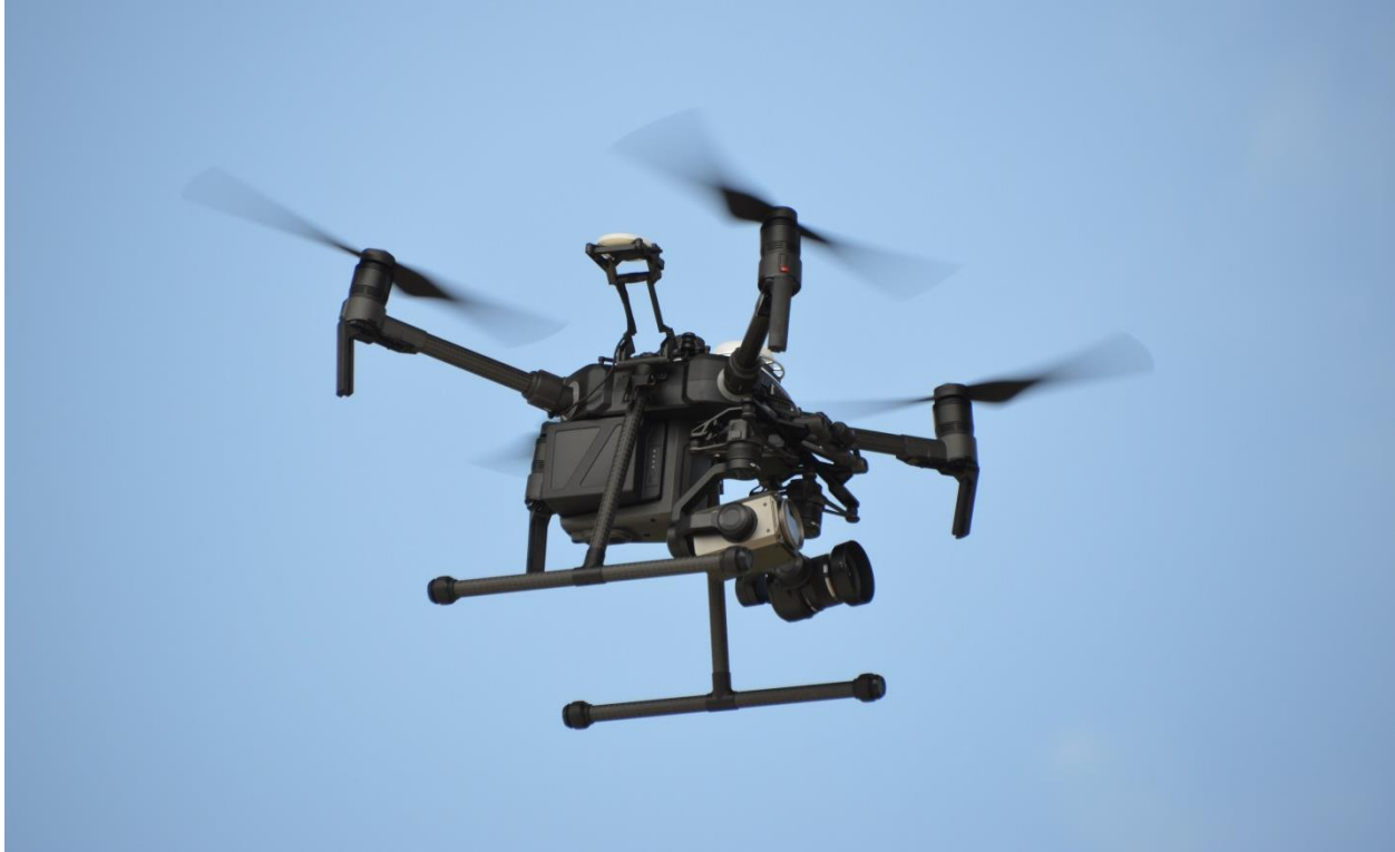
Figure 1. DJI Matrice 210 RTK in Air with Two Camera Systems Mounted to the Bottom
